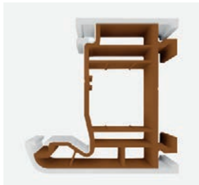
Co-extrusion technology facilitates a layered profile structure using recycled material. The photo shows a cross-section of a multilayer window frame.
